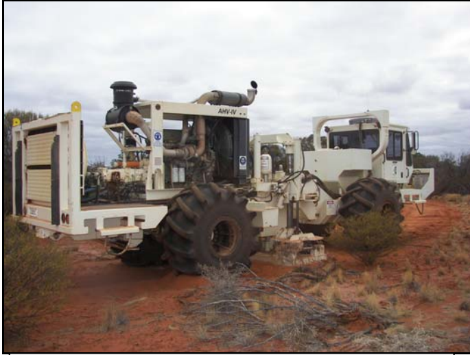
Vibrator truck suspended by vibrator plate.
